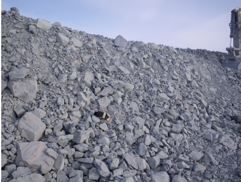
Photo 8: Quarry 2 – ROQ material from blast April 1, 2012. Very fine ROQ material with lots of fines.
